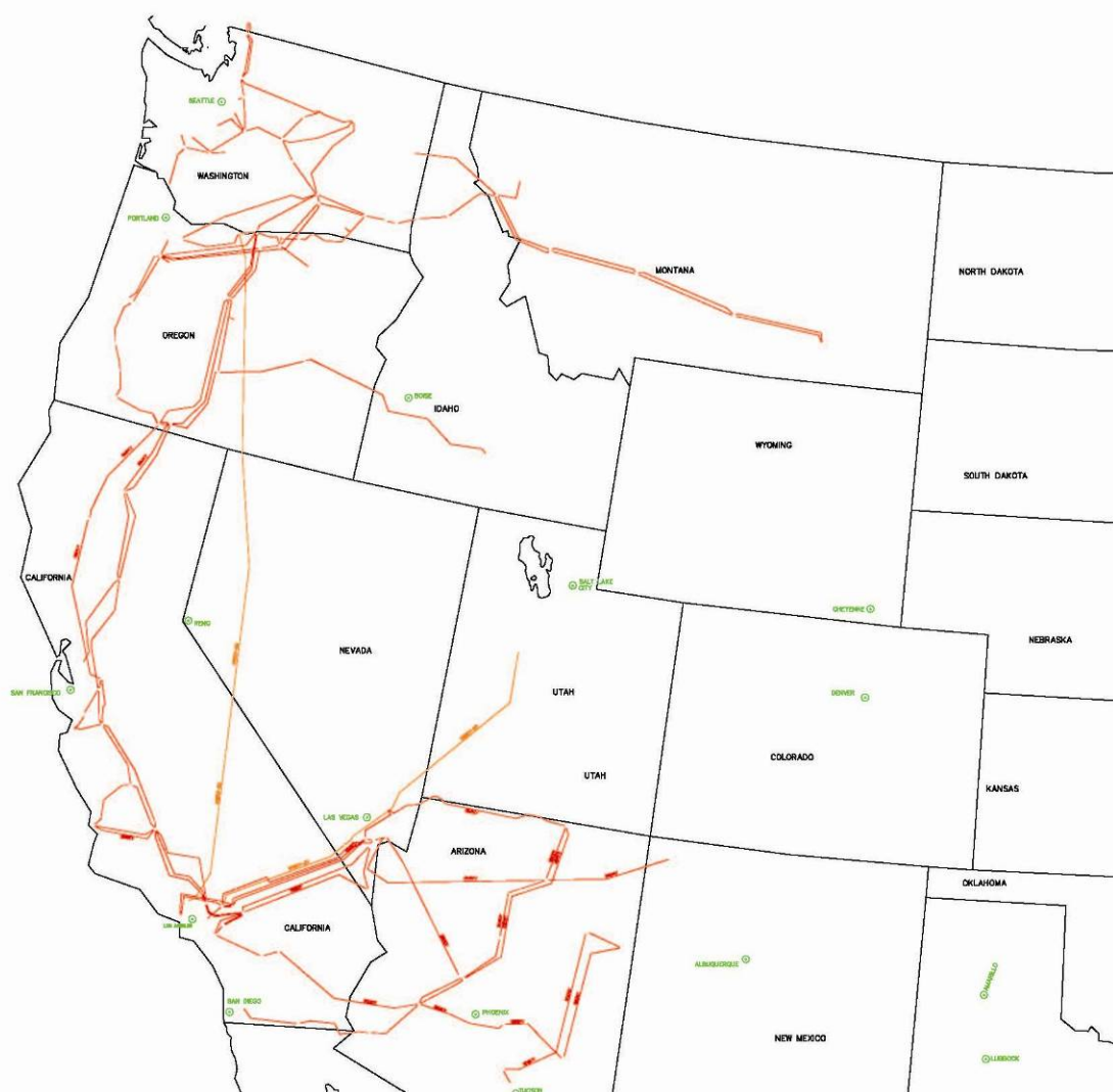
Figure 2-1 Extra High Voltage Transmission Network
